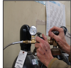
Fig. 38c Open filler hose slowly; pressure shown is pressure in small tank
