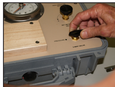
Fig. 24 Turn control valve to pressure
