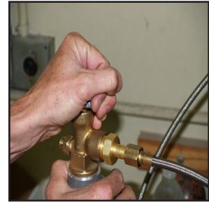
Fig. 38b Open valve just a little
