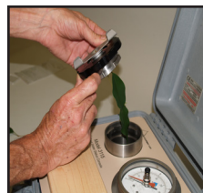
Fig. 22d Lower the severed leaf specimen into the pressure vessel
