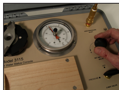
Fig. 25 Opening of metering valve
