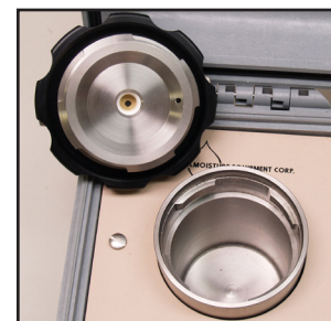
Fig. 3e Specimen holder with safety relief piston
