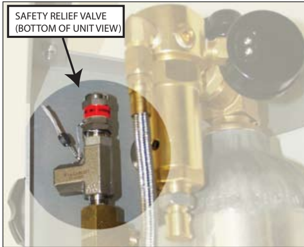
Fig. 11 - Safety relief valve
