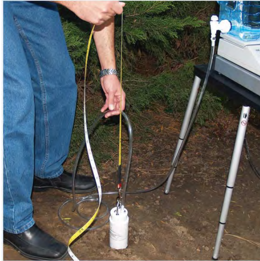
Fig. 16. Lowering RU and APM in borehole. Note do not hang from Tubing.
