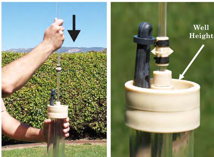
Fig. 26. Connecting Upper Air Tube to Middle Air Tube.
