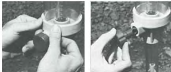
Fig. 37. Removing Reservoir Valve.
