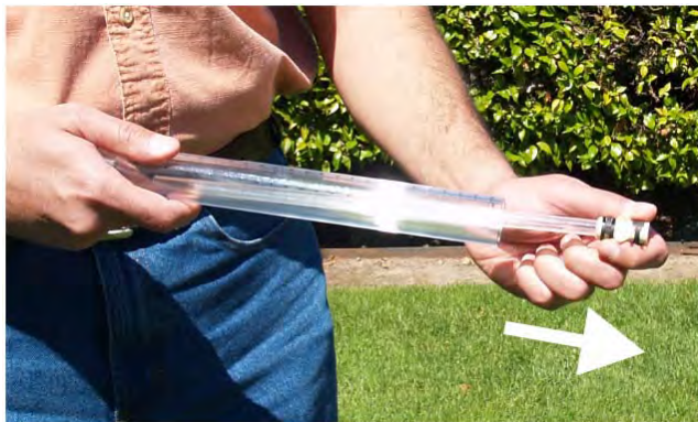
Fig. 25. Removing Upper Air Tube from Well Head Scale.
