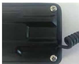
Sensor cable fed through the slot
