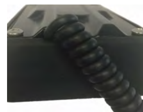
Sensor cable fed through the slot
