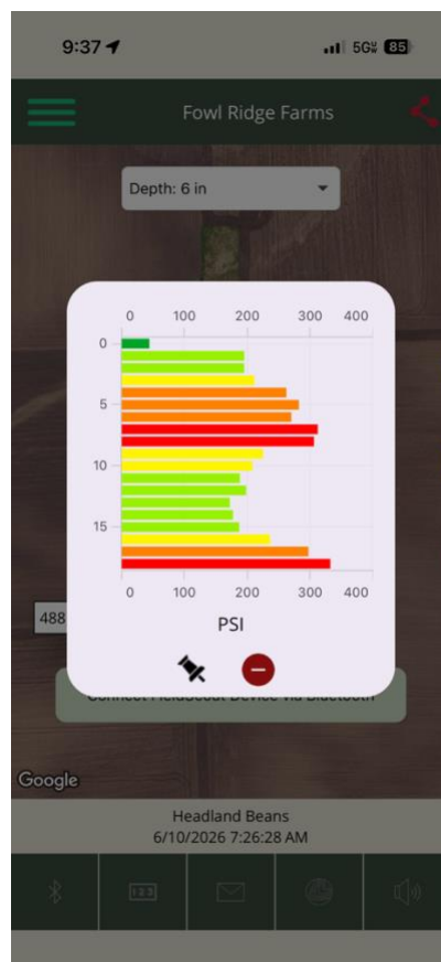
Compaction data at one measurement location showing PSI at 1" increments
