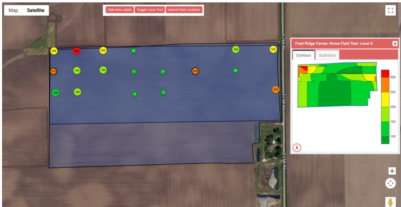
SpecConnect: Color-coded measurement points showing compaction at 6" depth across a field, with a corresponding heat map
